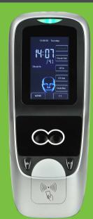
FAC700 is a new generation facial identification products, featuring standard functions with face recognition, PIN, and RFID verification. The unit encapsulates facial characteristics such as: relative position, size and shape of the eyes, nose, cheekbones, and the jaw features. All of these features are used for verification, and comparing with the enrollment data captured. The captured features are merged together into a value which are being compared to stored templates on the unit.
